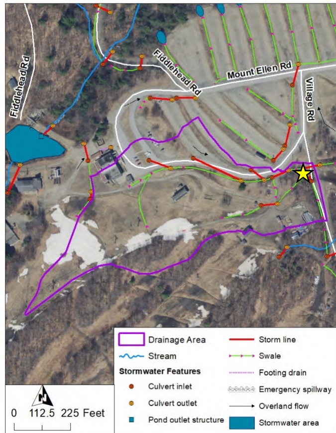
Figure 10. The drainage area for the Mt Ellen Rd and Village Rd site is shown outlined in purple. The location for the proposed infiltration basin is depicted with a yellow star.
