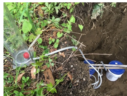
Figure 11. The Constant Head Borehole Permeameter Test in progress using a Johnson Meter.
